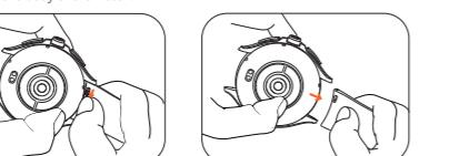
To assemble the strap: First place one end of the spring bar into the spring bar hole on the back of the watch, then pull back the quick release pin to insert the other end. After installation is complete, pull the strap to ensure that it is securely fastened.
